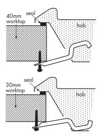
The screws should be tightened just sufficiently to secure the hob and pull the top pressing flush with the worktop.
